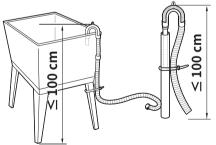
If the drain hose is too long, do not force it back into the appliance. This will cause abnormal noise. • When installing the drain hose to a sink, secure it tightly with string.
